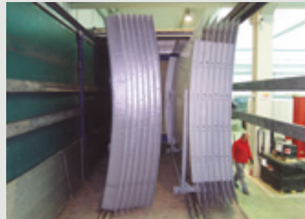
W-Tank® with H=11m, D=13.2m and 1,505m 3 capacity transported in a lorry.
